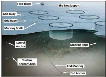
application of more or less even tension on all moorings to keep the grid taught. Tension will be maintained by using adequate moorings, anchor chains and anchors to suit seabed and hydrographic conditions and the dimensions of the system. Dark-coloured bird (top) nets will be used to protect the stock against bird predation throughout the life cycle. The existing shore-based facilities at Ballycrovane Pier or at Dinish Island, Castletownbere will to be used.
