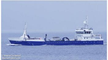
boat. These vessels will be used to transfer feed, equipment and crew and will have the capacity to carry out a wide range of day to day farm tasks including towing, anchor handling and net changing and cleaning. These vessels will operate from the shore base at Ballycrovane Pier/ Dinish Island where they will be moored when not in operation.
